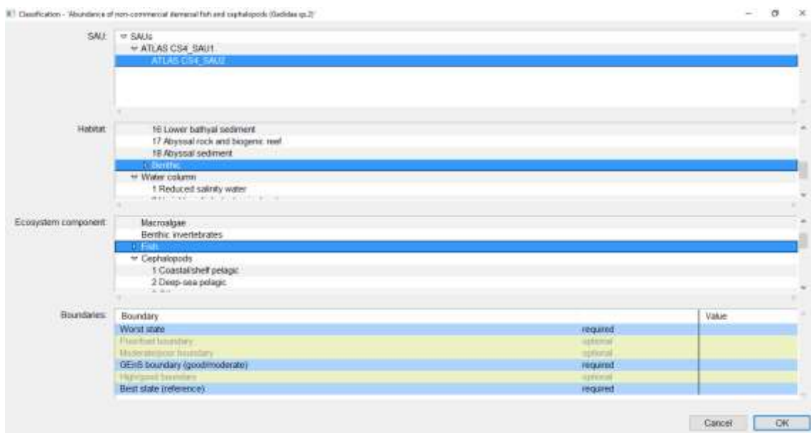
Fig. 12 NEAT screen to set-up the combining indicators with SAU, habitats and ecosystem components. For each of these combinations measured values and standard error as well as boundary values for the six predefined in NEAT categories of environmental status were set. Setup of boundary values for worst, good/moderate and best status are essential while for other categories, these are optional.
