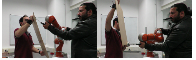
Fig. 7: Human operators teach the robot how to apply painting strokes.
