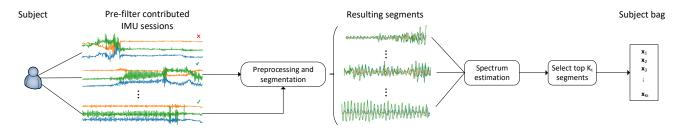
Fig. 1: Overview of the bag creation process. A single bag, that contains segments of contributed accelerometer signals, is created for each subject. The resulting bag is associated with a single tremor label, provided by domain experts.
