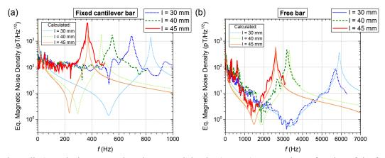
Fig. 7. (color online) Equivalent magnetic noise spectral density (EMND) measured as a function of the frequency in the long thin bar metglas / bidomain LNO composites (with length l = 30, 40 and 45 mm) operating in a: (a) fixed cantilever and (b) free vibrating regime. Superimposed are the results of the calculated EMND for the sensors with the
