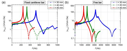
Fig. 5. (color online) Dynamic direct ME coefficients ( $|\alpha_{E31}|$ ) measured as a function of the field modulation frequency (with optimal bias fields of respectively H = 6.5, 3.5 or 2 Oe, for each length, and  $\delta H = 0.05$  Oe) in the long thin bar metglas / bidomain LNO composites (with length l = 30, 40 and 45 mm) operating in a: (a) fixed cantilever and (b) free vibrating regime.
