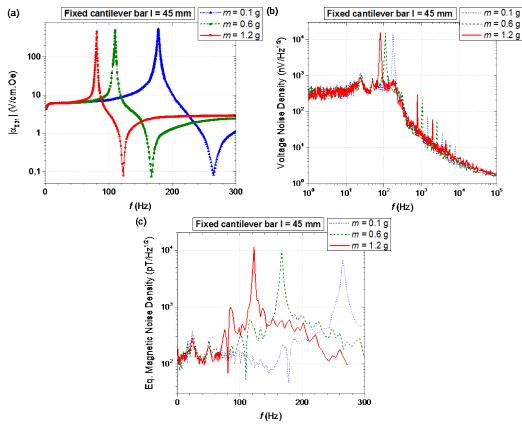
Fig. 8. (color online) (a) Dynamic ME coefficient (with H = 2 Oe and  $\delta H = 0.05$  Oe), (b) voltage noise spectral density and (c) EMND measured as a function of the frequency in the metglas/bidomain LNO fixed cantilever composite with length l = 45 mm and proof tip masses of m = 0.1, 0.6 and 1.2 g.
