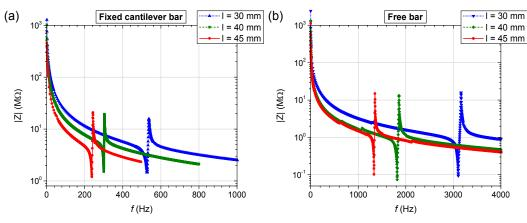
Fig. 3. (color online) Impedance spectra of the long thin bar metglas / bidomain LNO composites (with length l = 30, 40 and 45 mm) operating in a: (a) fixed cantilever and (b) free vibrating regime.
