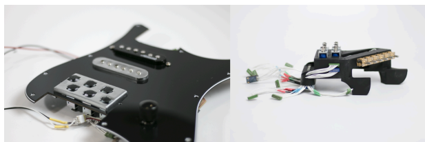
Figure 2: Two versions of our hardware design for inside mount (left) and outside mount (right).
