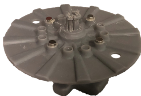
Figure 3: Magnets in Shielding Disk (only 4 shown)
