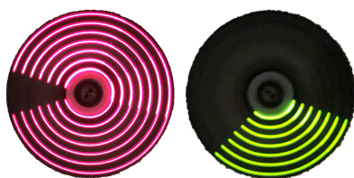
Figure 5: Two POV states taken at long camera exposure
