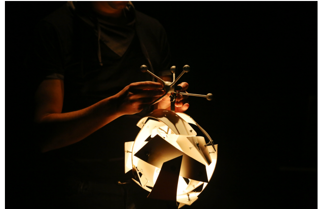
Figure 1: The light pendulum equipped with its passive infrared target.
