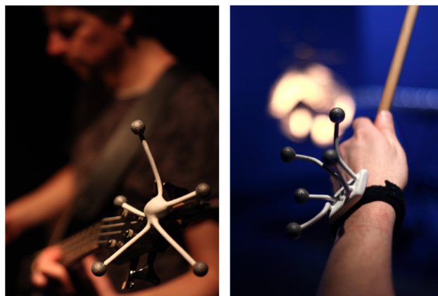
Figure 5: Left: target on bass guitar; Right: target on performer's wrist.
