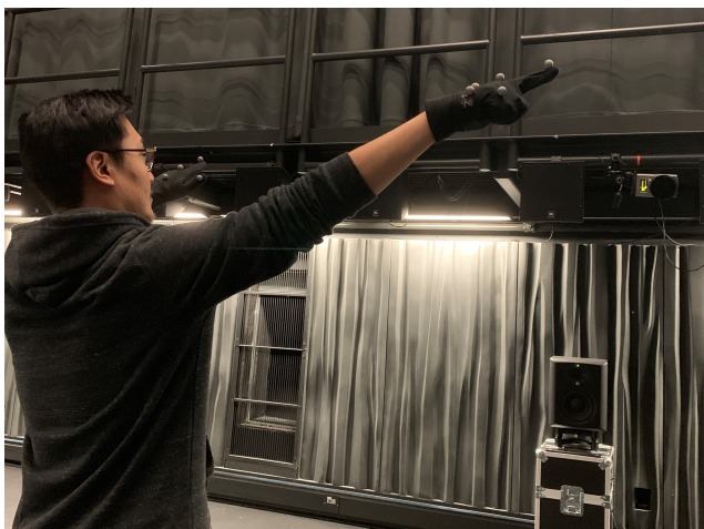
Figure 1: User manipulating the sound field using gloves fitted with retroreflective markers
