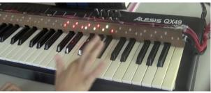
Figure 1. MIDI controller mounted with a LED stripe.
