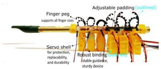
Figure 5. The overall design of flute device.
