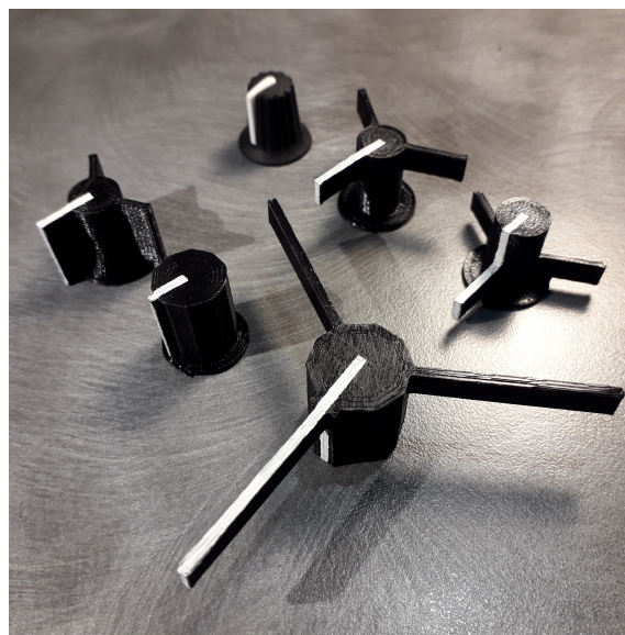
Figure 1: Alternative designs fabricated from PLA plastic filament alongside the original knob cap.
