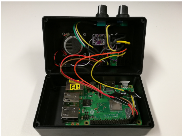
Figure 4: Hardware inside the enclosure. Hardware components consist of a Raspberry Pi, an analog-to-digital converter, two potentiometers, an audio amplifier and a speaker.
