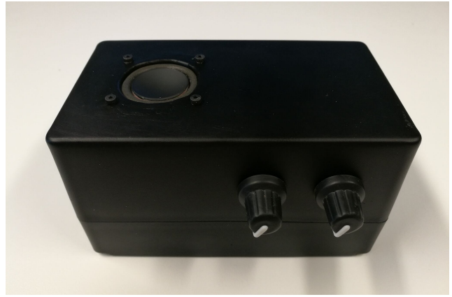
Figure 2: Close-up view of the physical intelligent instrument. The system has a built-in speaker and two knobs to control volume and sampling “temperature.”
