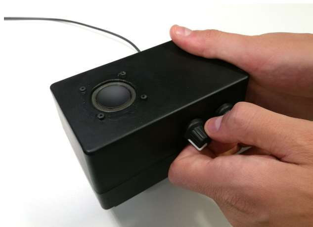
Figure 1: A user interacting with our physical intelligent instrument: a device that continually generates and performs music using a recurrent neural network. The system is self-contained with controls for volume and sampling “temperature” as well as a built-in speaker for sonifying generated notes.
