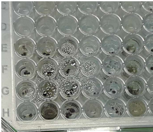
Data Figure 4. Example of condensation on the lid of a 96-well microtiter plate.
