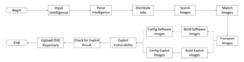
Fig. 2 Prototype system flow chart
