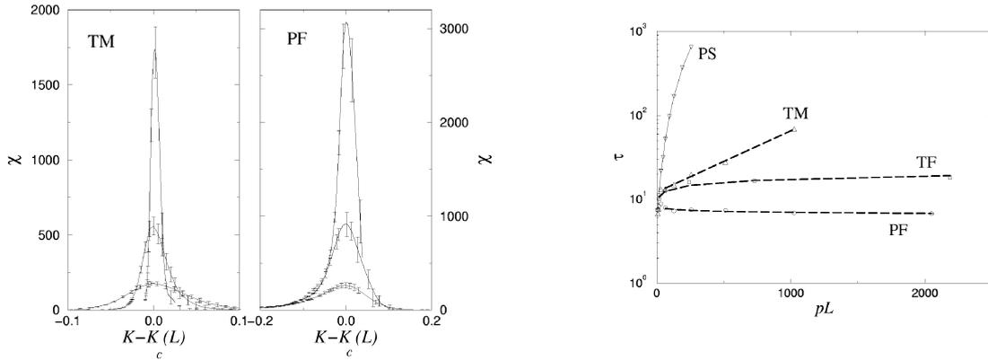
Fig. 1. Magnetic susceptibility  $\chi$  for TM ( $\delta$ -like asymptotic behaviour) and PF (power-law) (left) and size-dependence of the energy auto-correlation time which is expected to be exponential for a 1st phase transition and a power law for a 2nd order one (right).
