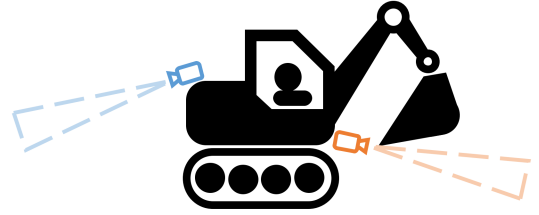
Fig. 1. Concept of sensing around a work machine using a non-overlapping multi-camera setup.
