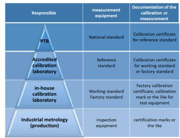
Figure 1 Calibration chain in Germany [3]
