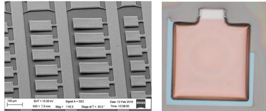
Fig. 1. Left SEM image of arrays of released GaN coupons on  $\langle 111 \rangle$  Si and Right transferred coupon bonded to intervia coated target substrate.
