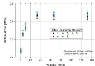
Fig. 2. Adhesion force as a function of velocity. 100x single measurements for each structure and each velocity.
