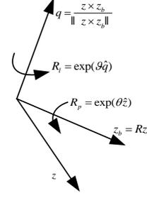
Fig. 2. The attitude of a rigid body can be represented by the attitude of a body-fixed axis, and the rotational motion around the body-fixed axis.
