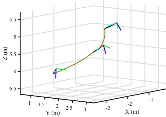
Fig. 4. The 3D snapshots from 5 s to 6 s. The cyan, green, and blue color line represent  $R_0e_1$ ,  $R_0e_2$ , and  $R_0e_3$  respectively. The red and black line represent link-1 and link-2 of the manipulator.
