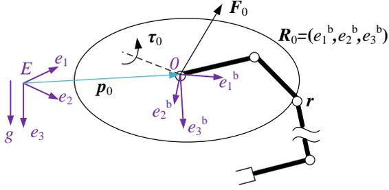
Fig. 1. Configuration of an aerial manipulator. The first joint locates at the COM of the aircraft base.  $F_0$  and  $\tau_0$  are expressed in the floating base fixed frame. The pose of link- $i$  of the manipulator is denoted as  $h_i \in SE(3)$ . The axis of joint- $i$  expressed in based fixed frame is  $z_i \in S^2$ . Note the COM of the base is not the COM of the entire system.
