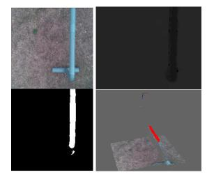
Fig. 7: Top images show the input frames from the Intel RealSense device. Bottom figures show respectively the argmax result from the CNN and the detection from the RANSAC algorithm, which highlight the result in red.
