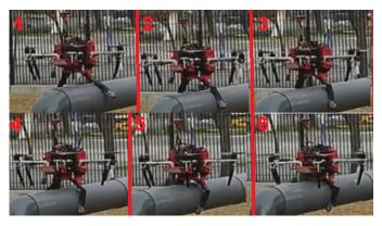
Fig. 9: Position estimation of the aerial platform related to pipe CS. This estimation is the result of the presented vision system and is used to perform the visual control of the robot.
