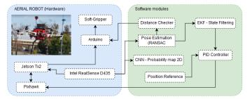
Fig. 1: Diagram of interactions between the hardware and software modules
