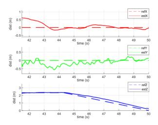
Fig. 10: Position estimation of the aerial platform related to pipe CS. This estimation is the result of the presented vision system and is used to perform the visual control of the robot.
