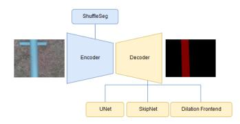
Fig. 6: Graph showing the Encoder/Decoder structure of the neural network used in this paper.
