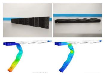
Fig. 5: The top left picture shows the limb printed; The top right picture represents the real profile; The bottom left picture is the displacement study; The bottom right picture shows the stress study
