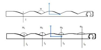
Fig. 4: The top image represents the symmetrical profile with the same angle and the same distance from the base. The bottom image has different angles and the distance to the base also changes
