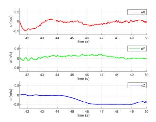
Fig. 11: Resulting control signals from the controller to the autopilot
