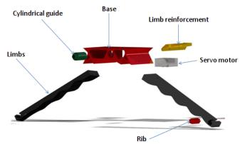
Fig. 3: Overview of the complete landing system. The two limbs can be seen, also the servomotor that applies the force to them. One rib is placed at the tip of each limb to distribute the forces and to reinforce the structure. The base is where all the components are attached. It is modular and easy to change thanks to the dovetail guides
