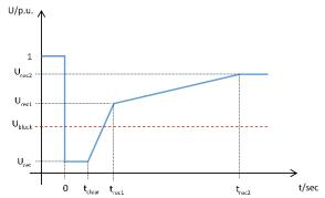
LVRT parameters for PE generators and HVDC:
