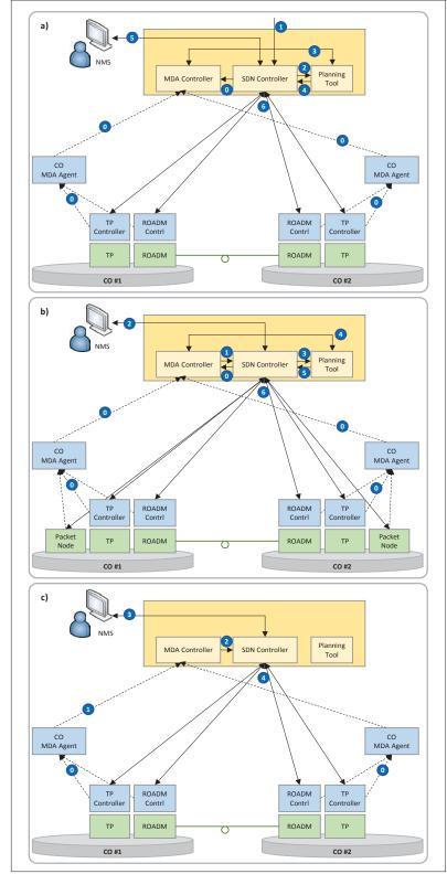
FIGURE 3. Control loops implementation: (a) lightpath provisioning with reduced margin; (b) dynamic network adaptation; and (c) lightpath degradation detection and modulation format adaptation.
