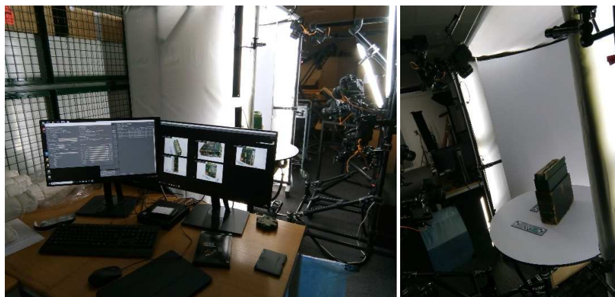
Views of BL digitisation station. Top complete view of the station equipment. Lower left the robocase system and the workstation controlling the image capture. Lower right turntable with the artefact being digitised.
