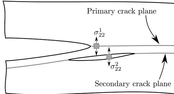
Figure 1: Illustration of the formation of multiple delamination cracks in a composite DCB specimen. The superscripts 1 and 2 refer to the primary and secondary crack planes, respectively.
