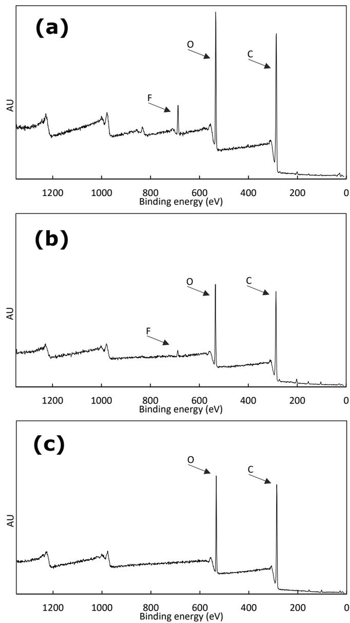
Figure 5: XPS spectra of treated and untreated fibres. (a) 100W DBD treatment, (b) 50W DBD treatment, (c) untreated
