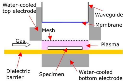
Figure 2: DBD treatment test setup
