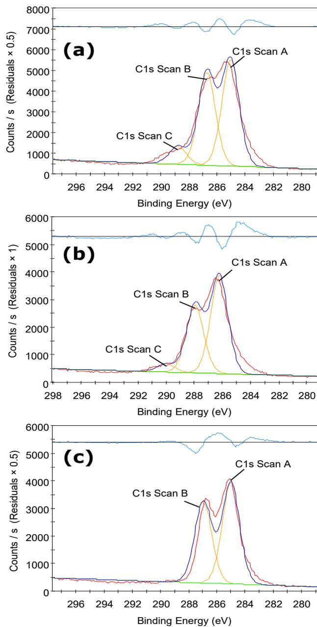
Figure 6: Typical C1s spectra of treated and untreated fibres. (a) 100W DBD treatment, (b) 50W DBD treatment, (c) untreated
