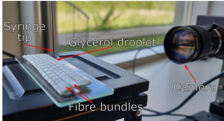
Figure 3: Contact angle measurement setup. (Full colour image available online.)
