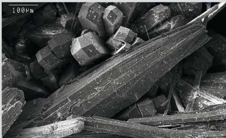
Curved ettringite crystals with phillipsite-Ca . Las Herrerías Quarry. J. Viñals coll and photo (SEM).
