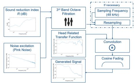
Figure 1. Block diagram algorithm of sound generation
