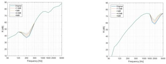
a. Massive wall with  $ETICS - f_0 = 250 \text{ Hz}$  b. Light wall with Gypsum 15 mm  $- f_0 = 2.5 \text{ kHz}$ Figure 3. Airborne sound insulation curves with simulated dip depth variations
