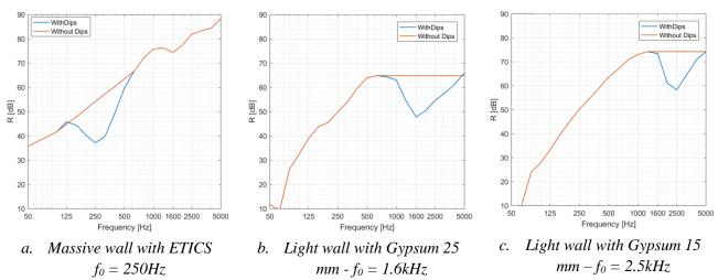
Figure 2. Measured airborne sound insulation of different walls with a mass-spring-mass resonance (a) or coincidence (b,c) dip and their equivalents after artificially removing the dip
