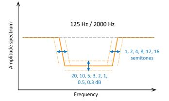
Fig. 1 Various combinations of width and depth of the notch filter used to prepare stimuli
