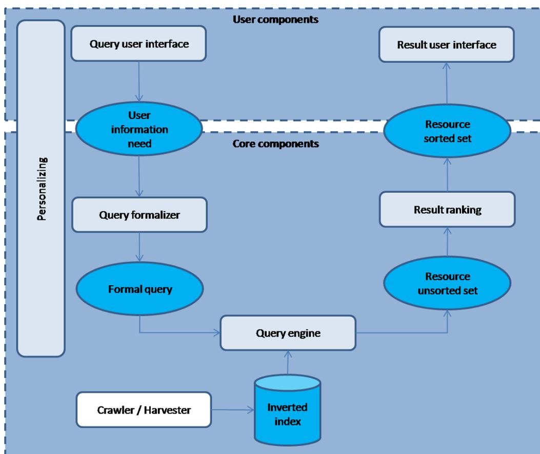
Figure 4.1: Typical IR system architecture
