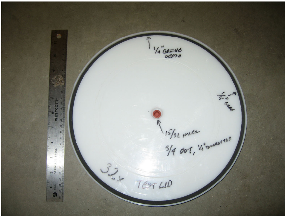
Figure 5. Lid, bottom view, with dimensions. Black ring is the silicone strip seal.
