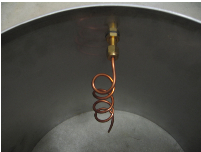
Figure 12. Inside view of a chamber vent.
