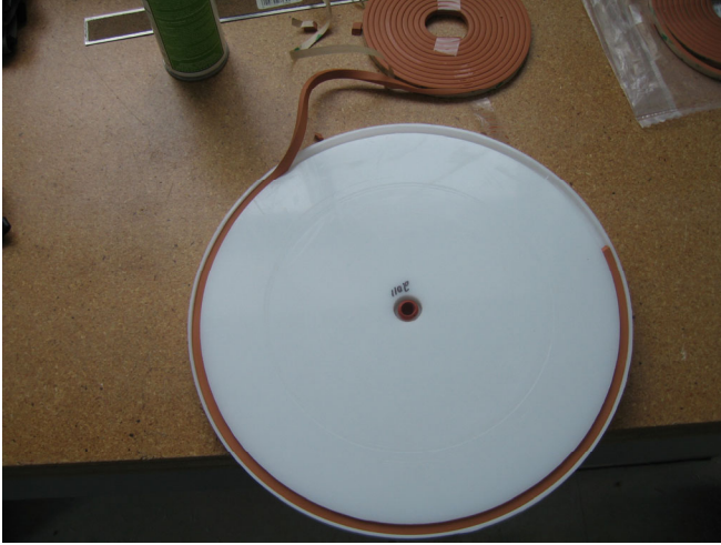
Figure 8. Seal installation into the lid groove on bottom surface.
