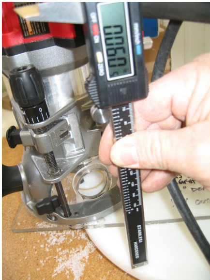
Figure 9. Groove in top surface of lid routed to \frac{1}{16} " (1.5 mm) depth.
