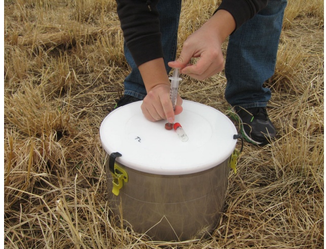
Figure 18. Chamber mixing and headspace sampling.
