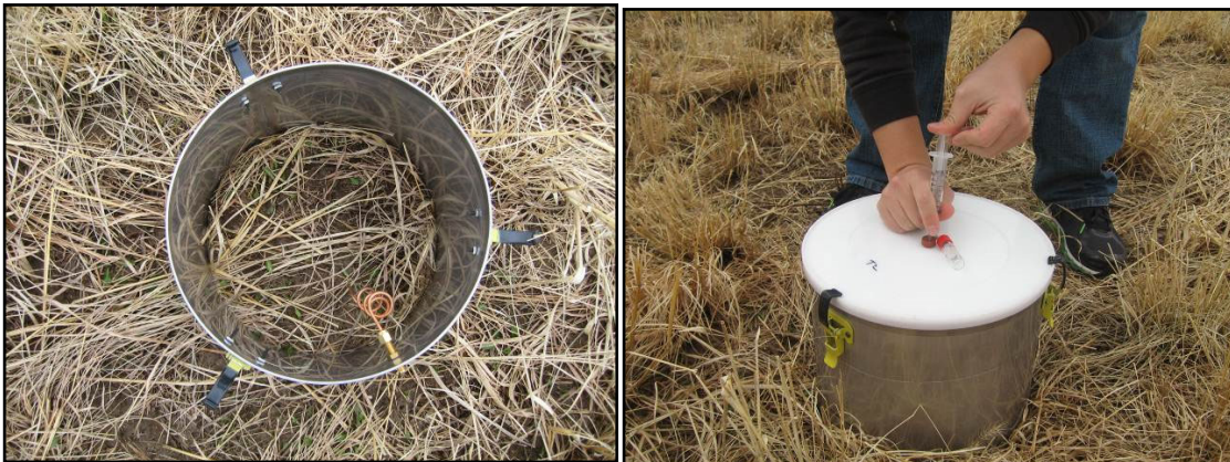
Figure 1. Static chamber as deployed in the field prior to (left) and during (right) gas sampling.
