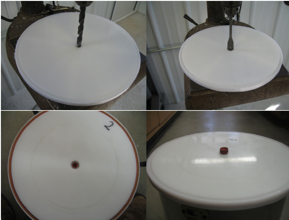
Figure 10. Installation of sampling septum.
