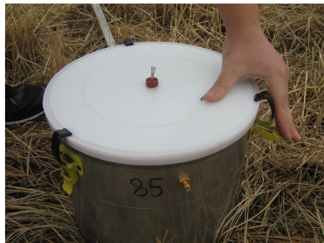
Figure 17. Chamber lid deployment using needle vent.
