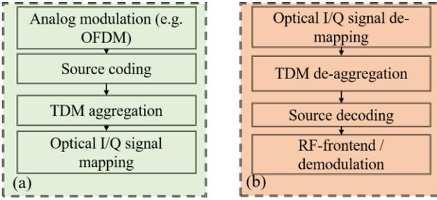
Figure 2. a) The transmitter flow and b) the receiver flow of proposed RoMCF system.
