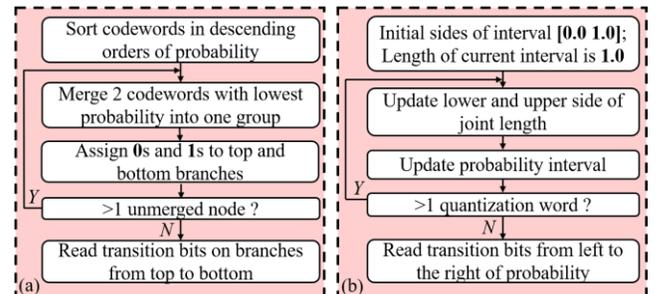
Figure 4. Lossless coding scheme with a) Huffman coding and b) arithmetic coding.
