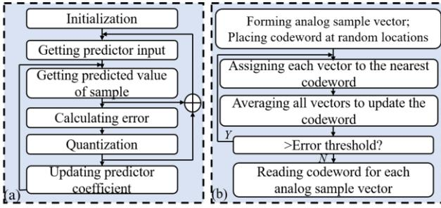
Figure 3. Lossy coding scheme with a) differential coding and b) vector coding.
