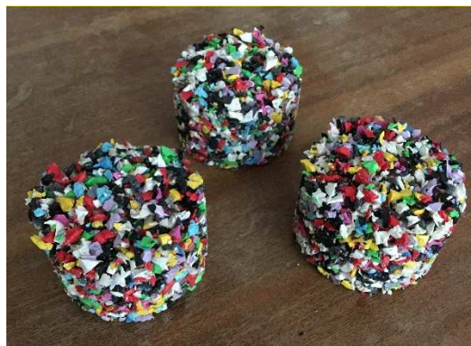
Figure 1. The reference sample (cylinders with diameter 10cm and height 6.5cm).
