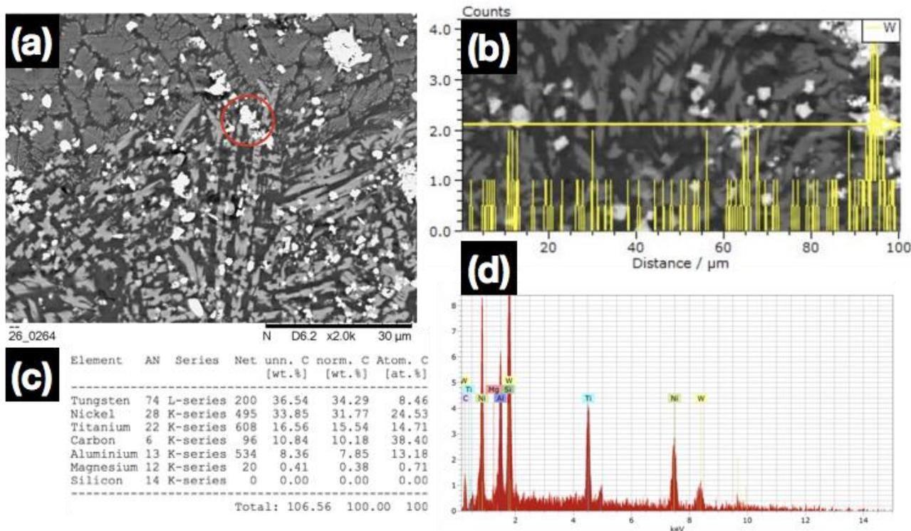
**Fig. 1.** (a) SEM micrograph of the coating middle section with visible intermetallics and particulates along with (b) EDX line scanning to identify WC particulates, (c) and (d) EDX elemental composition and spectrum for the inset in (a)
