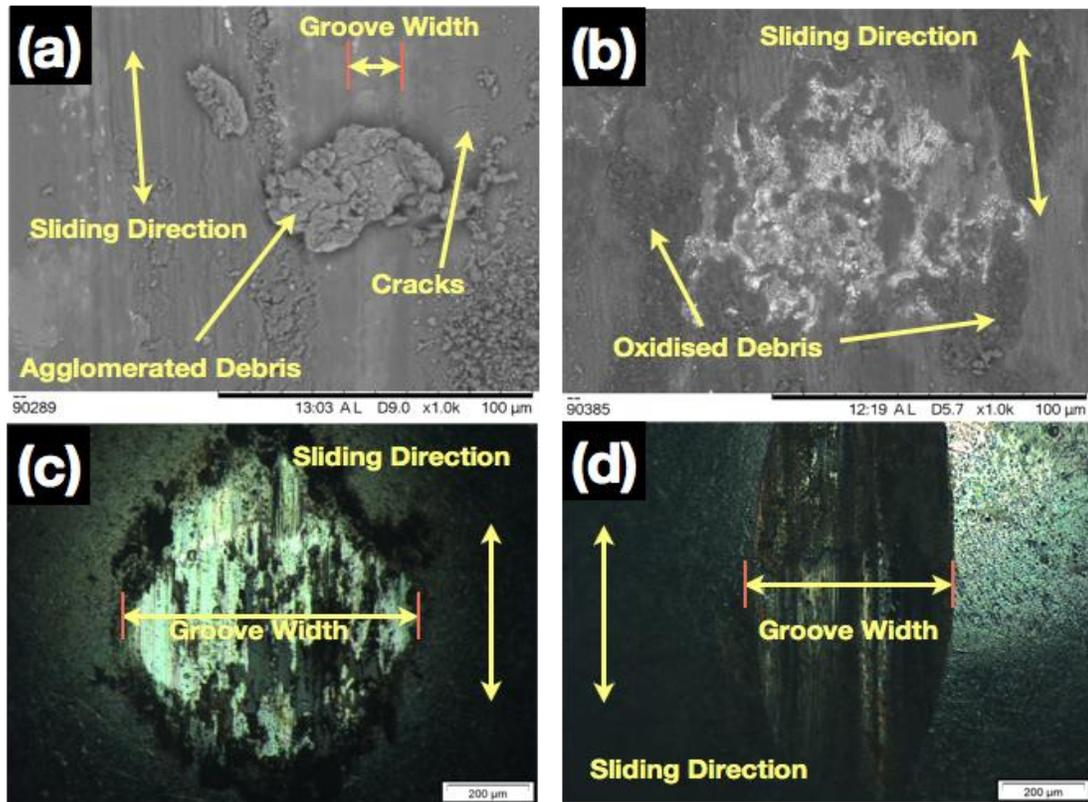
**Fig. 3.** SEM images of the worn scar for (a) AA5083 and (b) Ni-WC-TiO<sub>2</sub> in addition to the optical micrograph representing groove width for the counter-body of (c) AA5083 and (d) Ni-WC-TiO<sub>2</sub>
