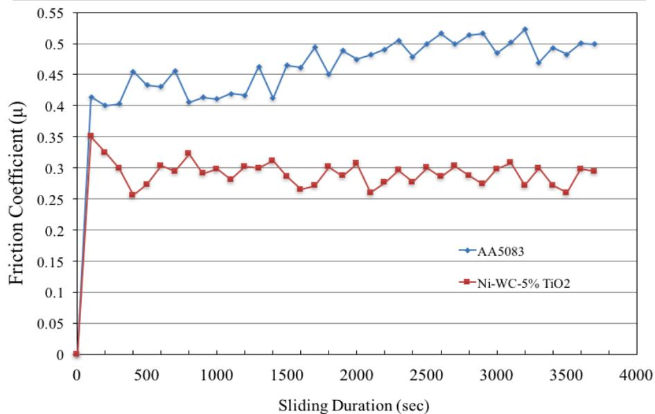
**Fig. 2.** The friction coefficient profiles for substrate AA5083 and the coating Ni-WC-TiO<sub>2</sub> for a duration of 1 hour
