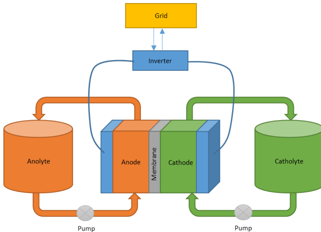
Figure 30: Basic concept of vanadium redox flow battery.
