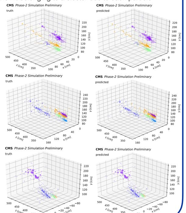
Displays of 3 example events. Points represent the HGCal hits, with size of the points proportional to the recorded energy at the sensor. Colors correspond to the source particle. The left plot of each row represents the ground truth, and the right plot shows the model prediction where hits are colored by the highest-probability cluster. The network architecture is based on GravNet, with some modifications with respect to the original implementation.
