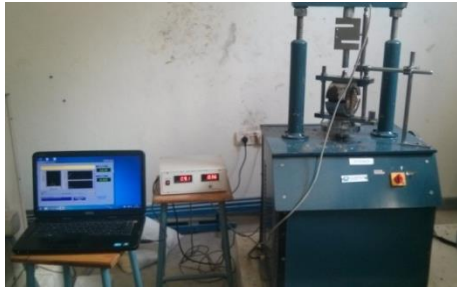
Figure 6. Marshall Test with Data Acquisition
