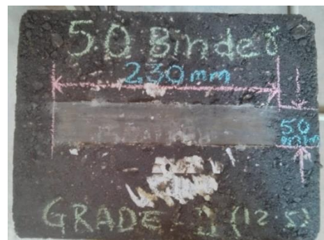
Figure 14. Rut Depth formation during Rut Test Figure 15. Position of Rectangular slab after Rut Test
