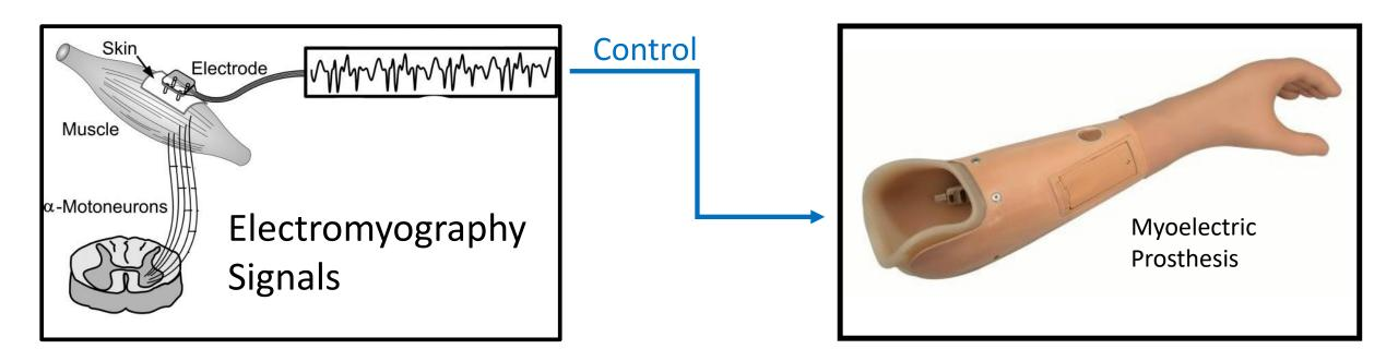
= "Decode" (motion-) intent from EMG signals and translate into motion of device
