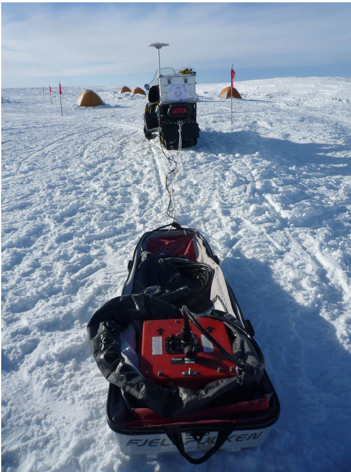
The GSSI antenna cable is connected and runs along the pulling rope. Make sure the sled is not pulled by the cable, but by the rope. A number of loops are made in the pulling rope to guide the
