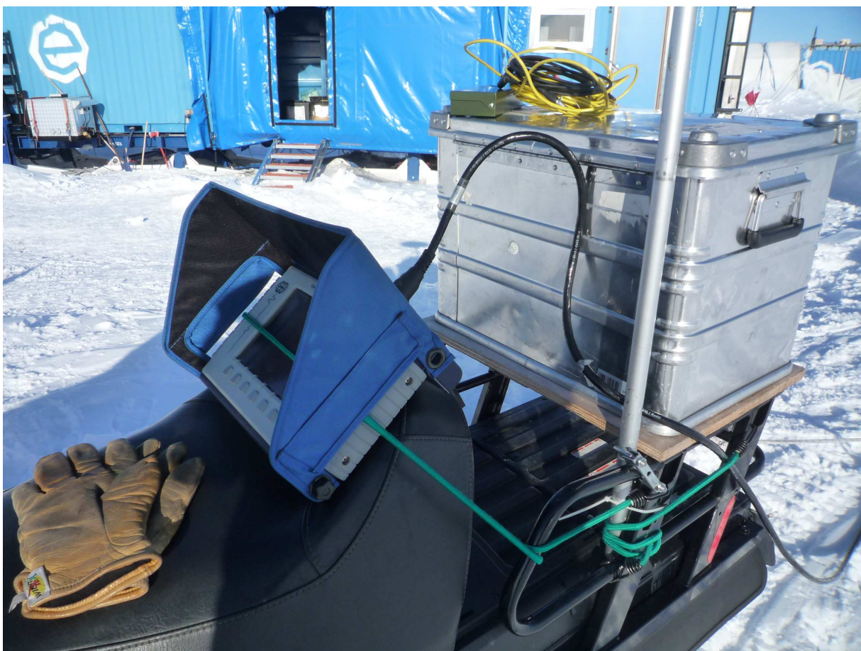
The GSSI instrument is fixed in place by an elastic strap.
