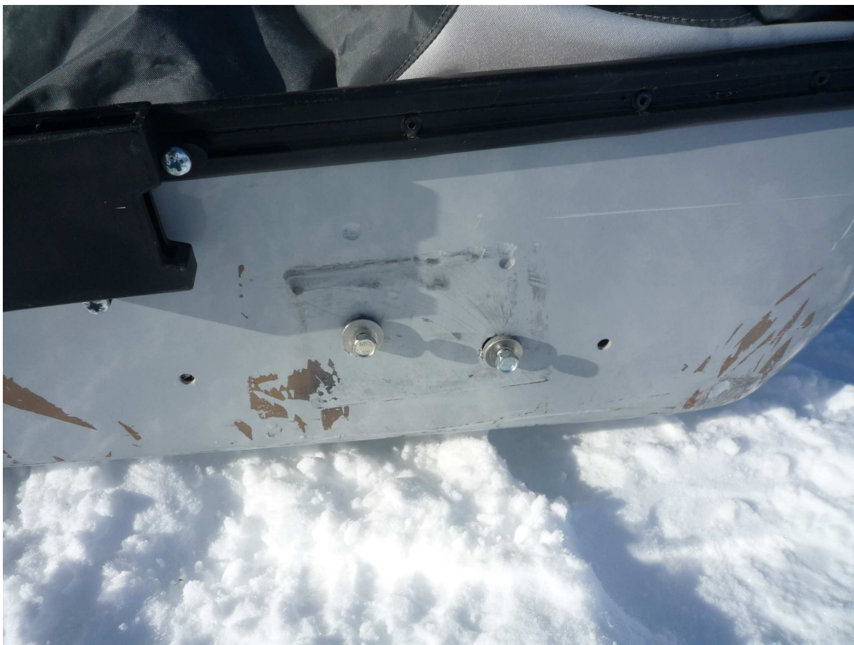
Two screws fix the little wooden block at the inside of the back of the sled (left side of the sled).
