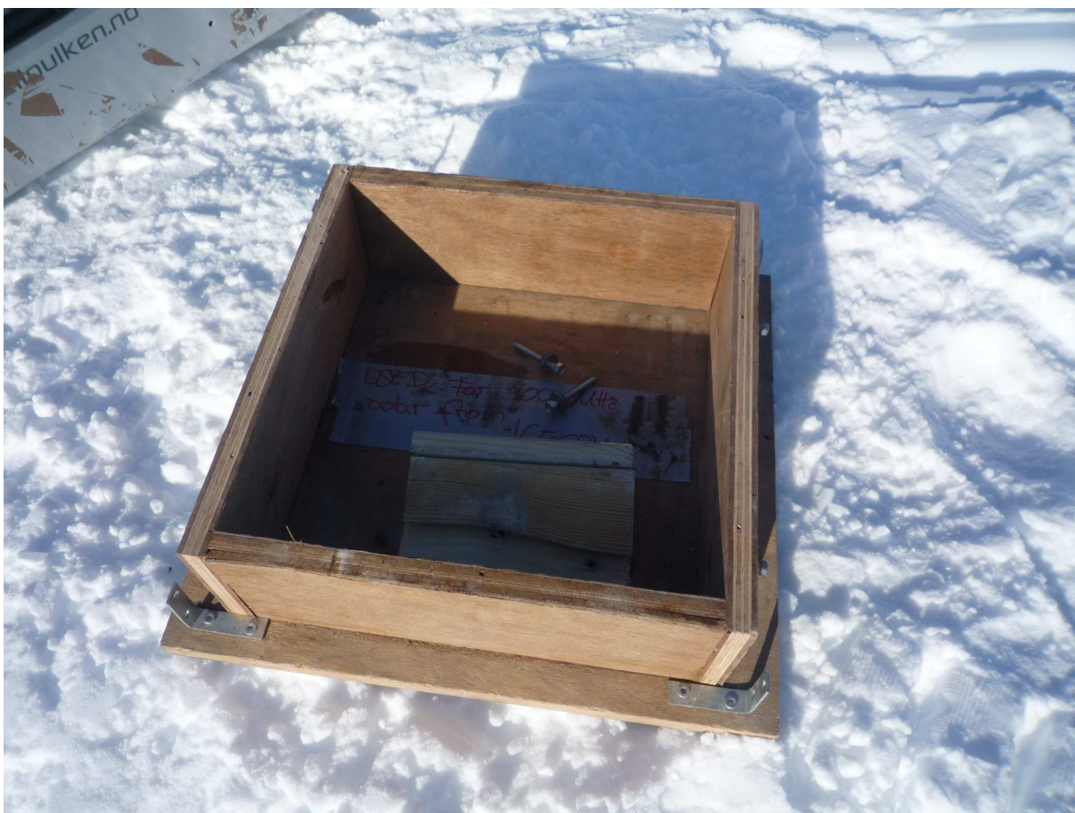
The radar antenna is put in a small wooden box (icecon written on it) that can be fixed in the small sled or the BELARE sled.
