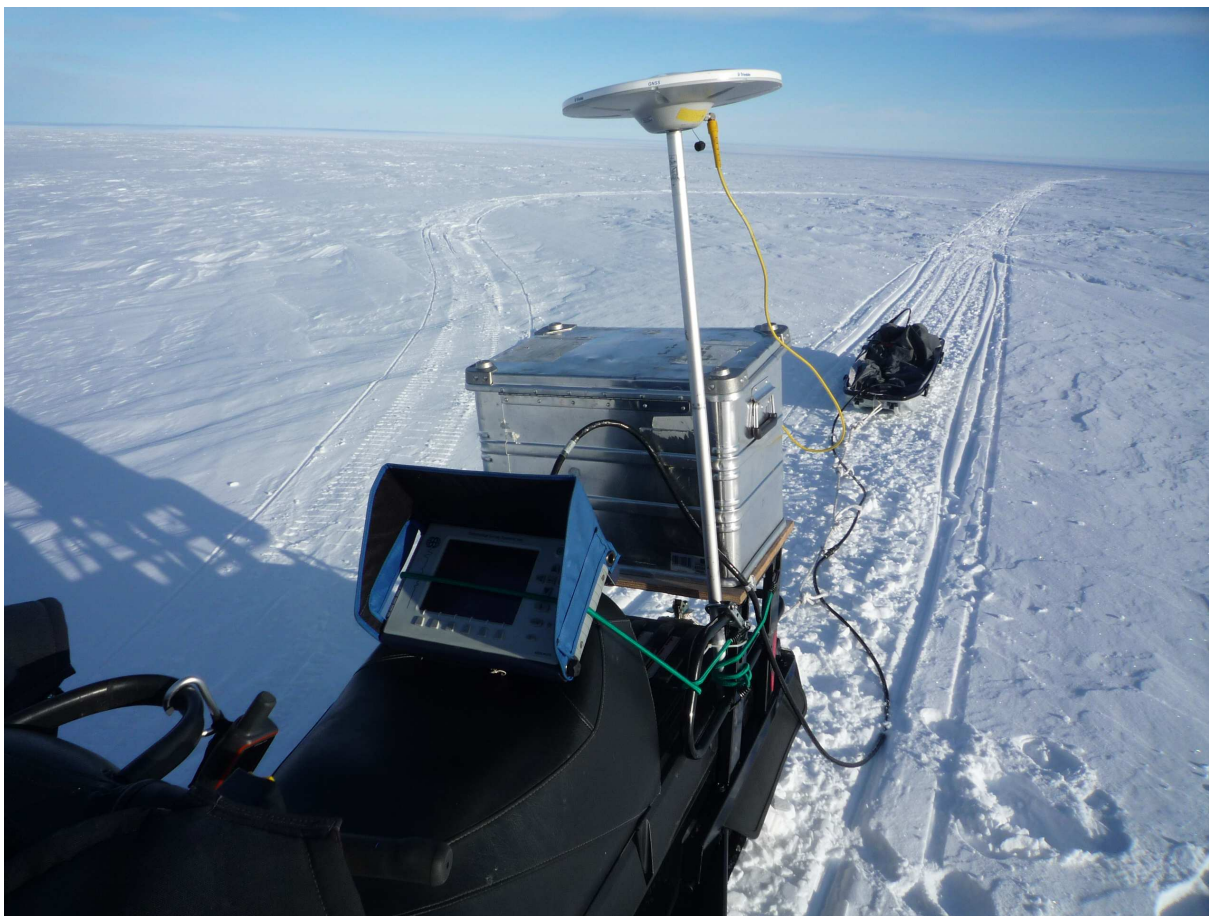
The GNSS antenna pole is fixed with u-bolt on the skidoo (a 550cc, not a 300cc) and further fixed with straps. The lid of the box is not closed so as not to squeeze the antenna cable. The GSSI cable runs along the skidoo and a rope to the small sled.
