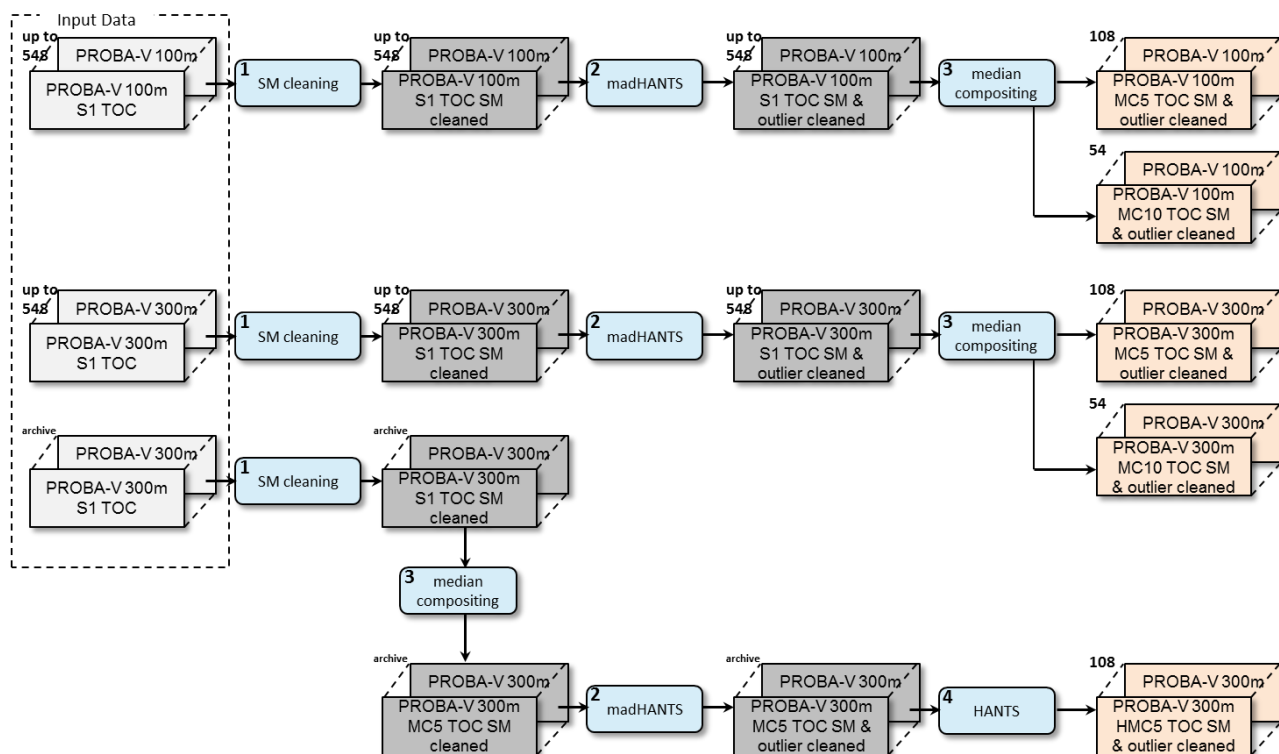
Figure 9: General overview of the data cleaning and compositing section in the CGLS LC100 product workflow. Note: Numbers in the upper left corner of data container indicate the number of layers - here number of observations.
