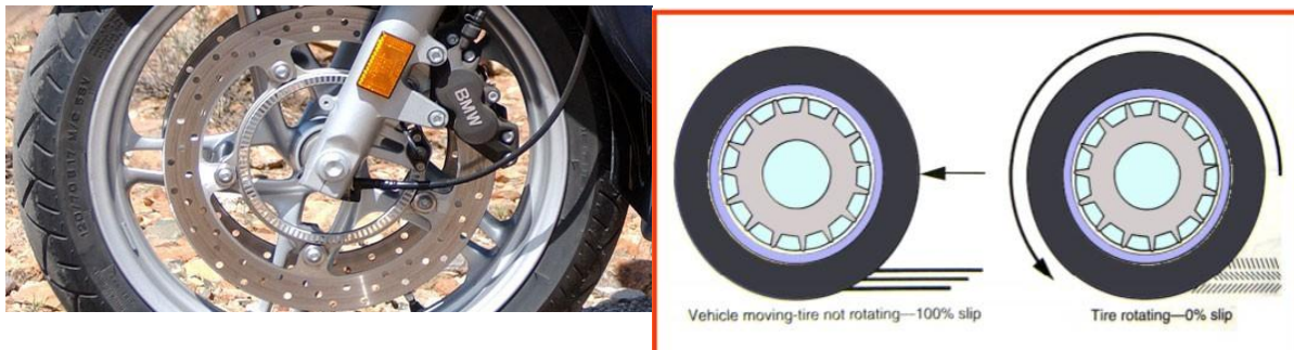
Fig. 1: ABS Breaks on BMW Motorcycle.
