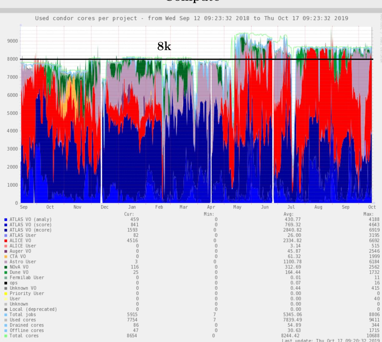
The HTCondor batch system allows usage of off-site machines. The  $\sim$  8k CPU cores (consisting of Intel and AMD (EPYC) processors) are distributed amongst the Institute of Physics (the Computing Center), the Faculty of Mathematics and Physics of the Charles University, Faculty of Nuclear Sciences and Physical Engineering of the Czech Technical University and CESNET. Usage by the experiments is based on fair-share.
