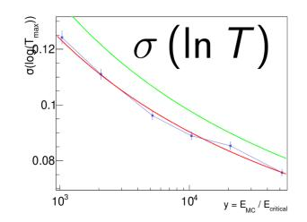
green line - GFlash parameters from arXiv:hep-ex/0001020 blue points - from full simulation on Pb red line - fit to full simulation (e.g. no Z dependency)
