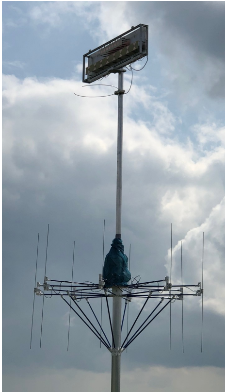
Fig. 4. VHF circular array with two linear arrays for 1 GHz and 2.4 GHz on top
