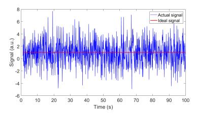
• **Noise always present**; even at steady-state reactor conditions, fluctuations due to e.g. vibrations of mechanical components occur
