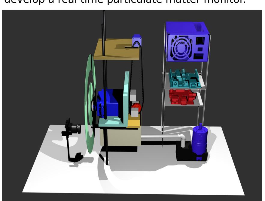
The monitor is based on low cost dust sensor coupled with chromatic modulation technique.
