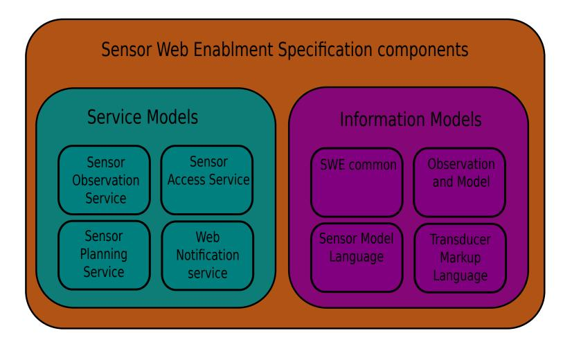
For example in Taiwan<sup>8</sup> Sensor Web Enablement specifications were used for managing heterogeneous sensors directed for debris flow monitoring. It organize and manages divers sensor resources such as Geophones, mobile and fixed monitoring stations for a coordinated functionality of risk preparedness and disaster management.
