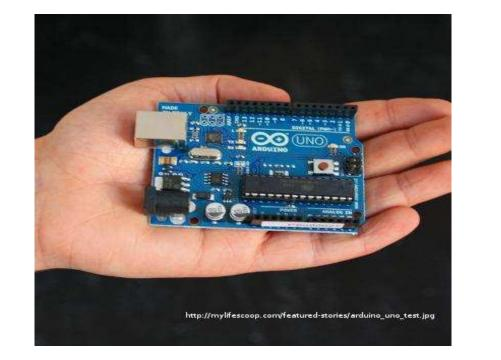
Inexpensive and easy usability makes them one of the rapid prototyping and development tools especially related with sensing and monitoring requirements.
