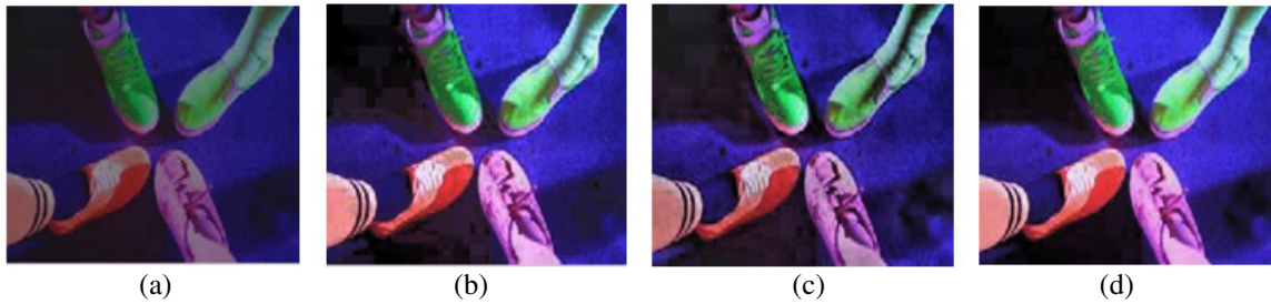
Fig 5. Enhancement results of Shoe image: (a) Original, (b) HE, (c) CLAHE, and (h) ESIHE
