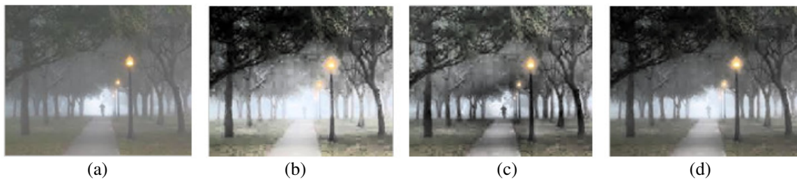
Fig 6. Enhancement results of Forest image: (a) Original, (b) HE, (c) CLAHE, and (h) ESIHE
