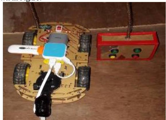
Figure18 CCD Camera and 3G SIM Router Combined with Spy Robot
