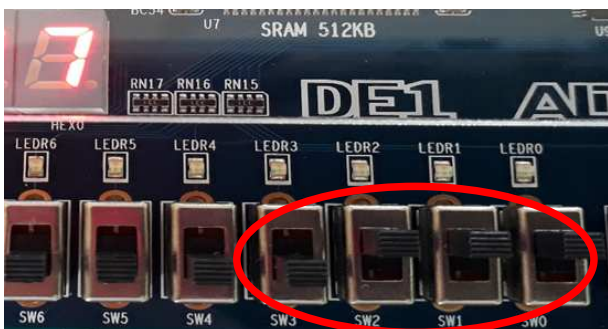
Fig14. Decimal Value 7 on 7Segment for Binary value '0111'
