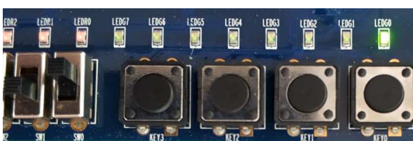
Fig32. T input '1' and Clock input '1' (At The 7 th Positive edge of Clock)
