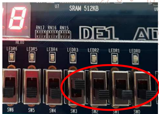
Fig15. Decimal Value 8 on 7Segment for Binary value '1000'
