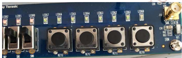
Fig23. Condition of Clock=1 and Input D=1
