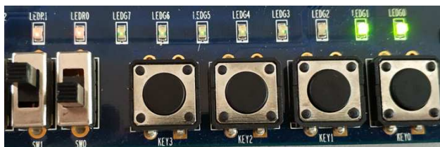
Fig30. T input '1' and Clock input '1' (At The 5 th Positive edge of Clock)
