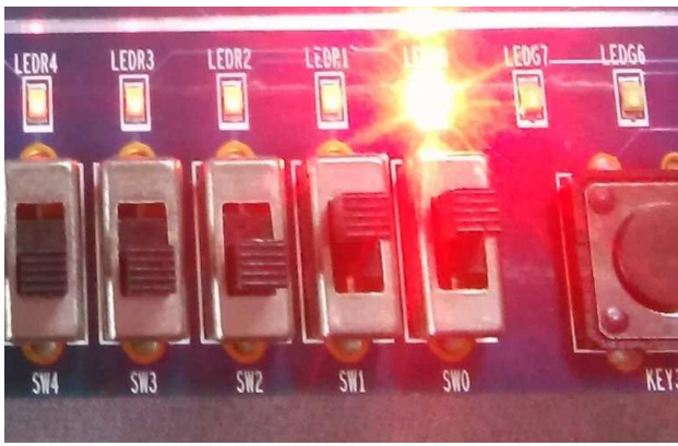
Fig5. Output LED is OFF when Inputs are '11' condition
