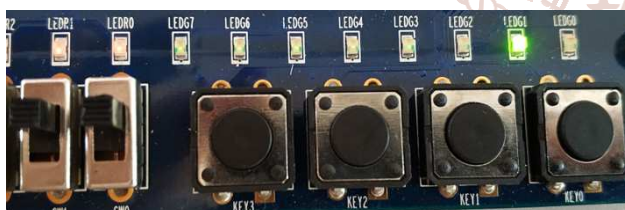
Fig31. T input '1' and Clock input '1' (At The 6 th Positive edge of Clock)
