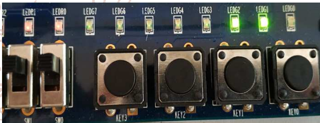
Fig27. T input '1' and Clock input '1' (At The 2 nd Positive edge of Clock)
