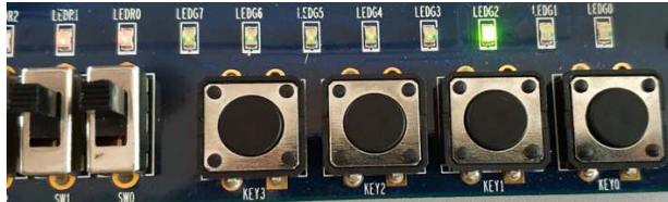
Fig29. T input '1' and Clock input '1' (At The 4 th Positive edge of Clock)
