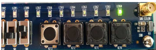
Fig21. Condition of Clock=1 to 0 and Input D=1
