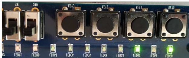
Fig28. T input '1' and Clock input '1' (At The 3 rd Positive edge of Clock)
