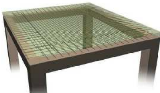
Figure5: Two-Way Simply Supported Slab.
