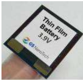
Fig.2.3: Thin film Lithium Nanotech rechargeable battery
