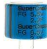
Fig.2.2: Super capacitor for storing large energy density charges from energy harvesting
